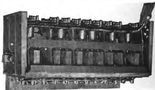
Fig. 4664. Unit Switch Group for Electro-Pneumatic System of Multiple Control. Westinghouse A. C. Electric Locomotive.
